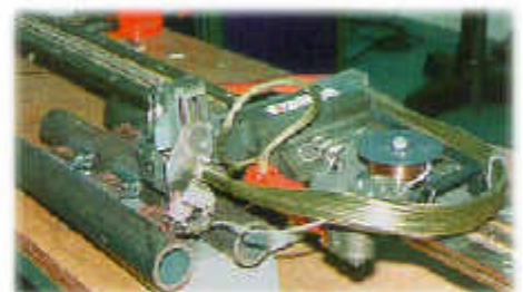
Polycar on rail for longitudinal welding
