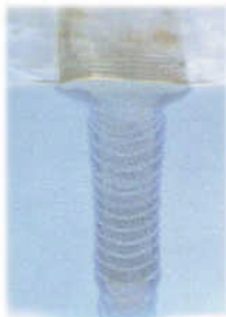
Macro of a narrow TIG-hotwire weld (50 mm wall thickness)
