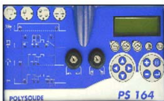
Control panel for operator / PS 164
